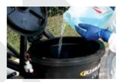
The Hypro Cleanload eliminates the need for operators to climb on and around machines while handling expensive and dangerous chemicals.
